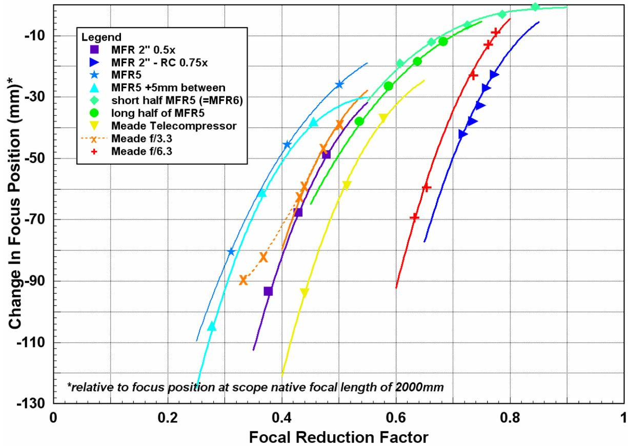
Figure 4 Simple FR Measured Focus Position Change vs. Focal Reduction Factor
