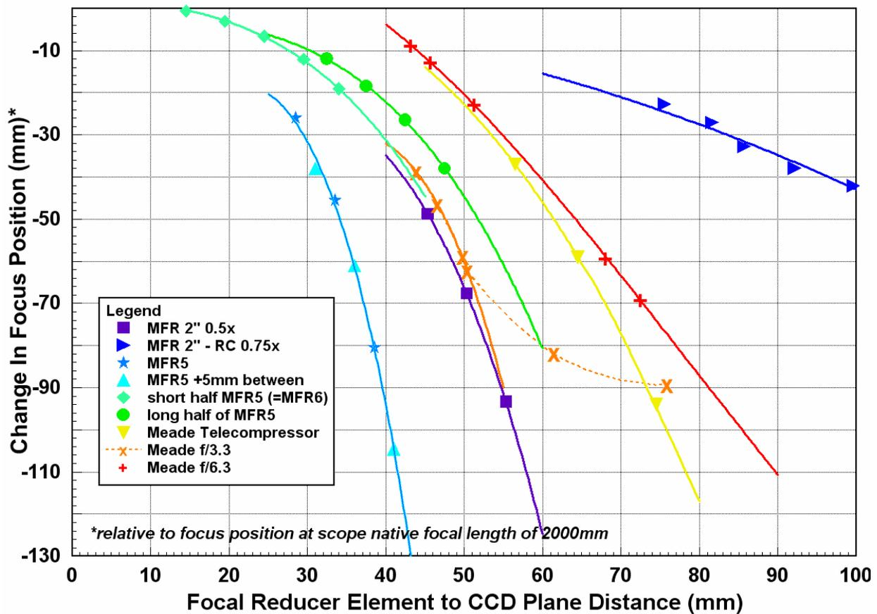
Figure 3 Measured Focus Position Change vs. FR-to-CCD Distance
